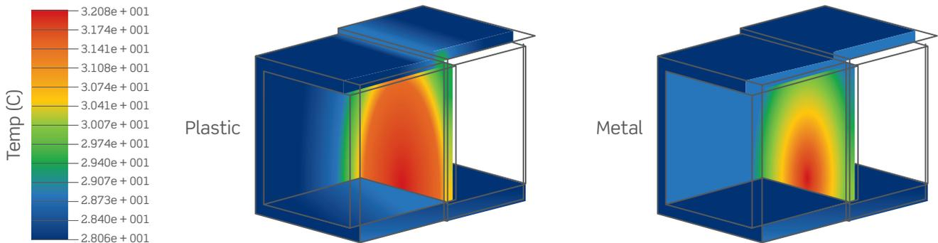
**Figure 6:** Thermal simulation of jack bodies using plastic and metal
