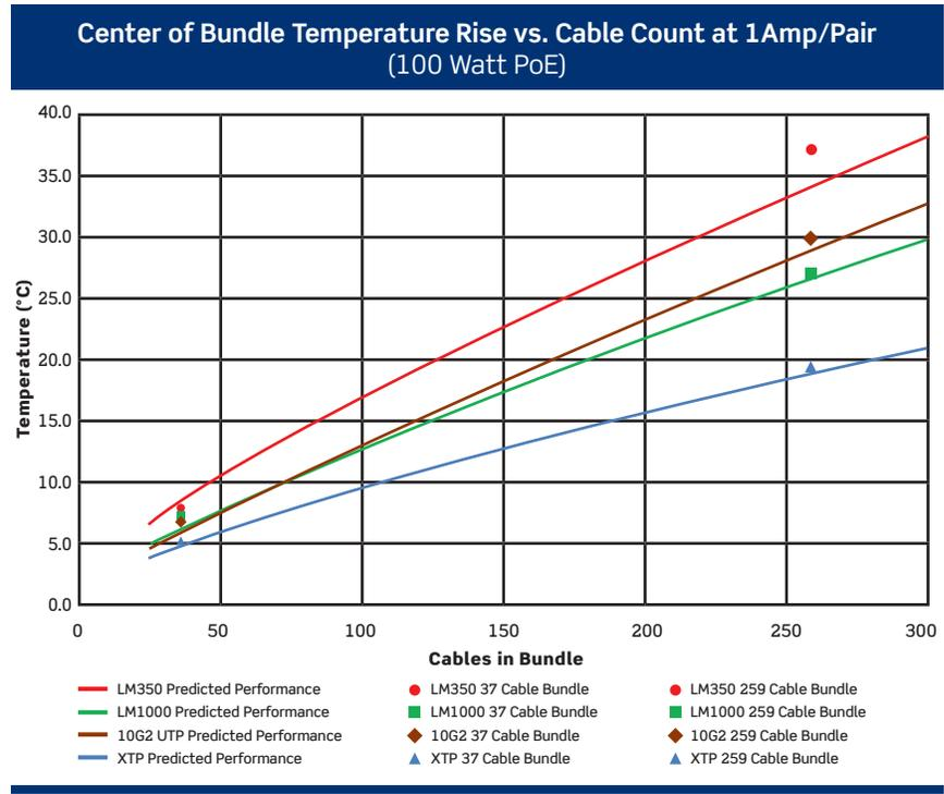
**Figure 5:** Modeled vs. measured temperature rise of innermost cable in bundle in an open tray.
